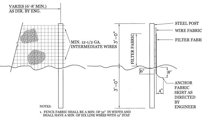
2. FABRIC SHALL BE FOR EROSION CONTROL AND MIN. OF 36" IN WIDTH. FABRIC SHALL BE FASTENED ADEQUATELY TO THE WIRE FABRIC AS DIRECTED BY THE
