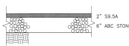
NOTE: PAVEMENT SECTION MAY VARY DEPENDING UPON FIELD CONDITIONS. CONTRACTOR SHALL COORDINATE w/ OWNER & GEOTECHNICAL ENGINEER TO DETERMINE ACTUAL PAVEMENT SECTION.
